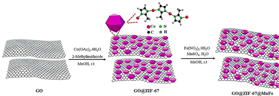
**Scheme 1.** Schematic illustration of the synthetic process for GO@ZIF-67@MnFe.
